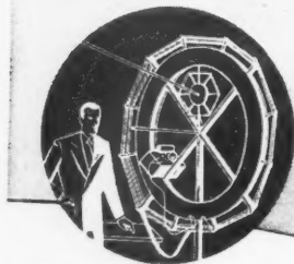
1920 Loop antenna for 400-500 meter ship-to-shore radio telephone receivers. Its design enabled earliest measurements of field strength.
